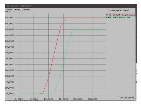
The above figure shows the comparison of throughput which is amount of data received at the destination node in the network. The values of the throughput for the proposed scheme at 260 Kbps are higher than the existing scheme at 210 Kbps indicating better performance of the network.
