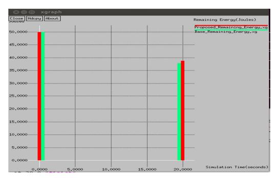
The above figure shows the comparison of the energy consumption for both the schemes. Initial energy of 50 joules was provided to the nodes. By applying the 3 conditions defined earlier in the work, the remaining energy for the proposed scheme has been found to exhibit more values at 39 Joules as compared to existing scheme having value at 37.5 Joules.
